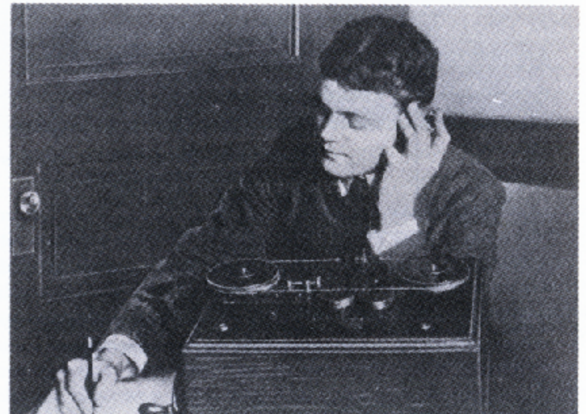
Fig. 5.22 A Marconi hysteresis detector in use [Collins, A.F. 'Manual of Wireless telegraphy', (Wiley/Chapman & Hall, 1906) p.165]
